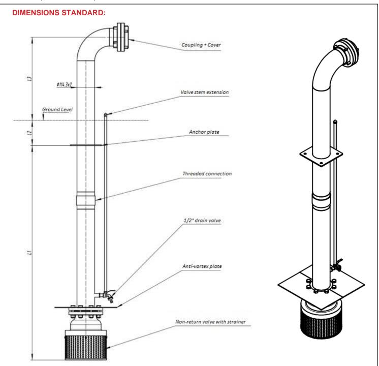
In the order, specify dimensions L1, L2, L3 and or if the pipeline route is different from the standard one (exit through the chamber wall and not through the cover, etc.) send a drawing or sketch showing the dimensions and pipeline route.
